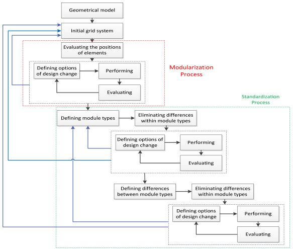
Figure 1: Working in Level 1- Building geometry
