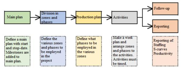
Figure 1: Overview of the Integrated Planning concept
