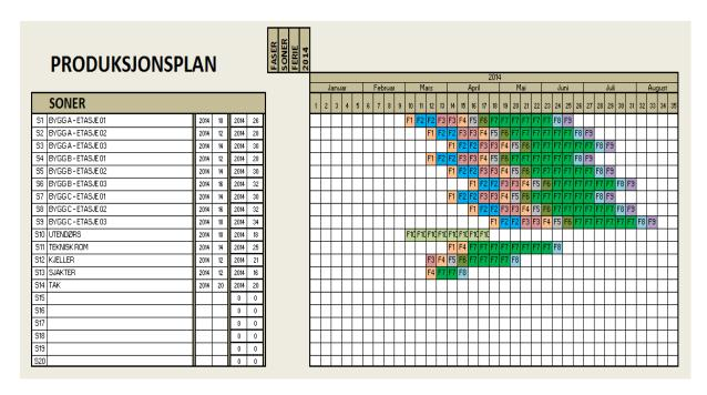
Figure 2: Location-based production plan
