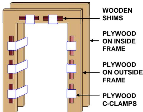
Figure 10: Diagram of Plywood Fix
