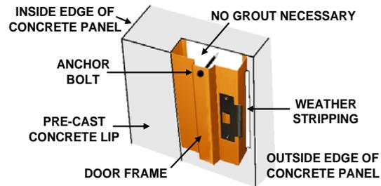
Figure 11: Concrete Lip Fix
