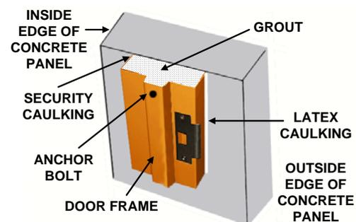
Figure 3: 3-D Diagram of Frame Design
