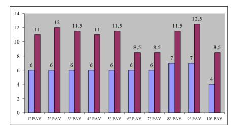
*Figure 4: Production graphs for first ceiling rendering coat – duration and number of mortar batches in each story.*
