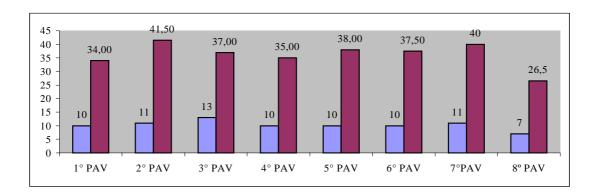
*Figure 5: Production graphs for final ceiling rendering coat – duration and number of mortar batches in each story.*
