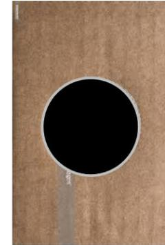
Cardboard with circular hole in between of 50mm on a piece of size of A4 sheet.
