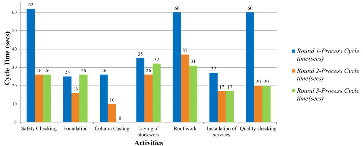
Figure 13. Cycle time comparison of each trade for each round
