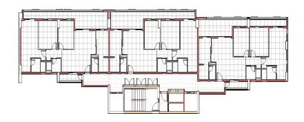
A residential high standard building of a single tower with two garage floors, 15 typical floors and 1 roof. It has three apartments per floor, with approximately 90 m<sup>2</sup> each.
