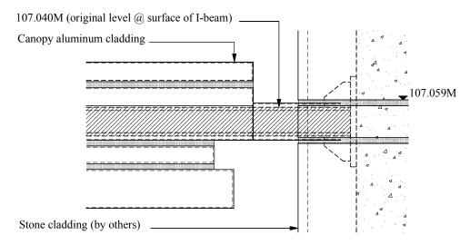
Figure 3: Front View @ Steel I-Beam Fixing Area
