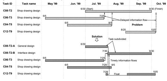
Figure 6: Process of CPM Enhancement
