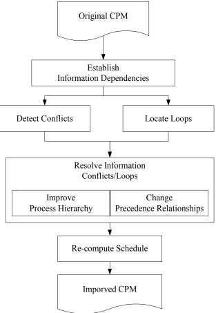
Figure 1: Structure of IFIPM
