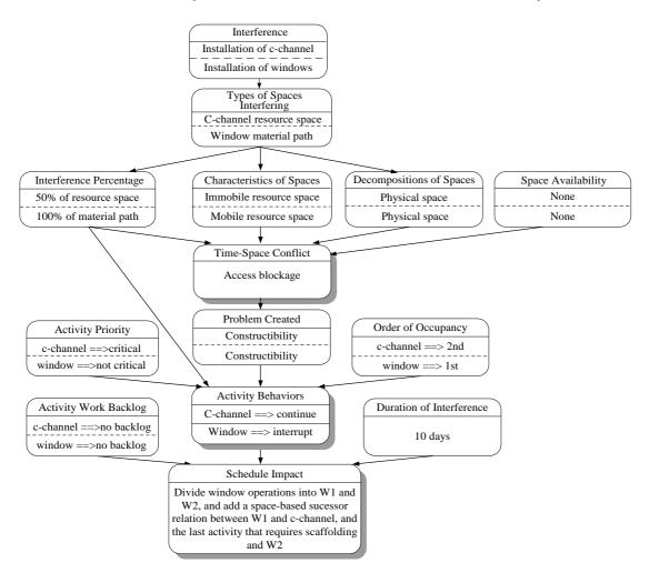
Figure 6: Application of the initial time-space conflict analysis framework for conflict between c-channel and window installation in the sample case
