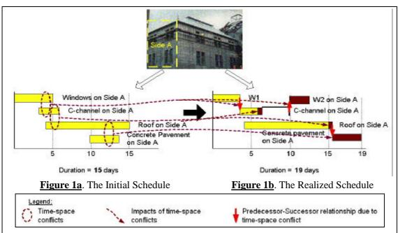
The sample case focuses on the execution of four activities on side A of the building. An initial three-week look-ahead schedule with a target duration of 15 days has been developed prior to construction. Due to the time-space conflicts between window and c-channel installation, c-channel and roof installation, and roof and concrete pavement installation, the initial schedule cannot be executed as is:
