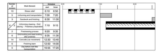
Figure 5: Standardized Work Combination Table of roof tiles production work elements.
