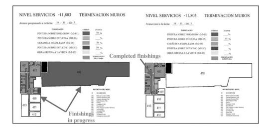
Figure 5: Visual Control and Tracking of Finishing Activities (Detection and Solution of Delays)
