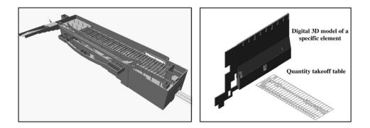
Figure 1: A Digital 3D Model of the Subway Station and the Quantity Takeoff of Concrete
