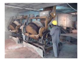
Concrete-mixer that produces the pre plaster at the construction site.
