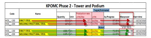
Figure 5: Completion report highlighting the differences between the originally planned manpower requirements versus the actual
