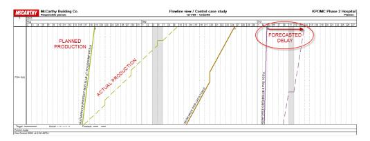
Figure 3: The forecasted delay of reinforcing due to staging conflicts between pier cap rebar and waterproofing
