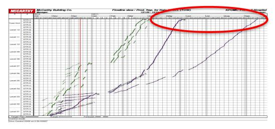
Figure 6: The flowline on 12/2012 showing 3.5 months delay in welding completion based on current production rates
