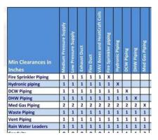
Figure 5: Sample clearances for building systems coordination used in early design (Source: Andy Sparapani, HerreroBoldt)
