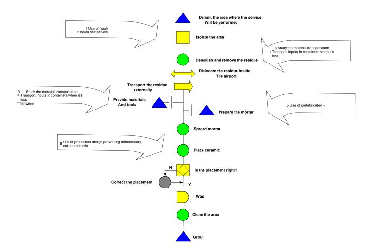
Figure 2: Flowchart of the replacement of ceramic coating in the construction process
