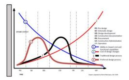
Figure 1: Preferred design process and traditional design process comparing (Graphic originated by Patrick MacLeamy, AIA / HOK)
