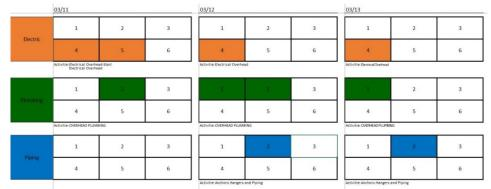
Figure 2: Example output for 3 days of work for 3 trades for a 6 zone floor plan
