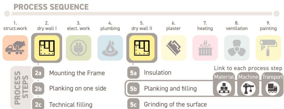
Figure 2: Example sequence with application of the resource categories to the work steps for dry wall construction.
