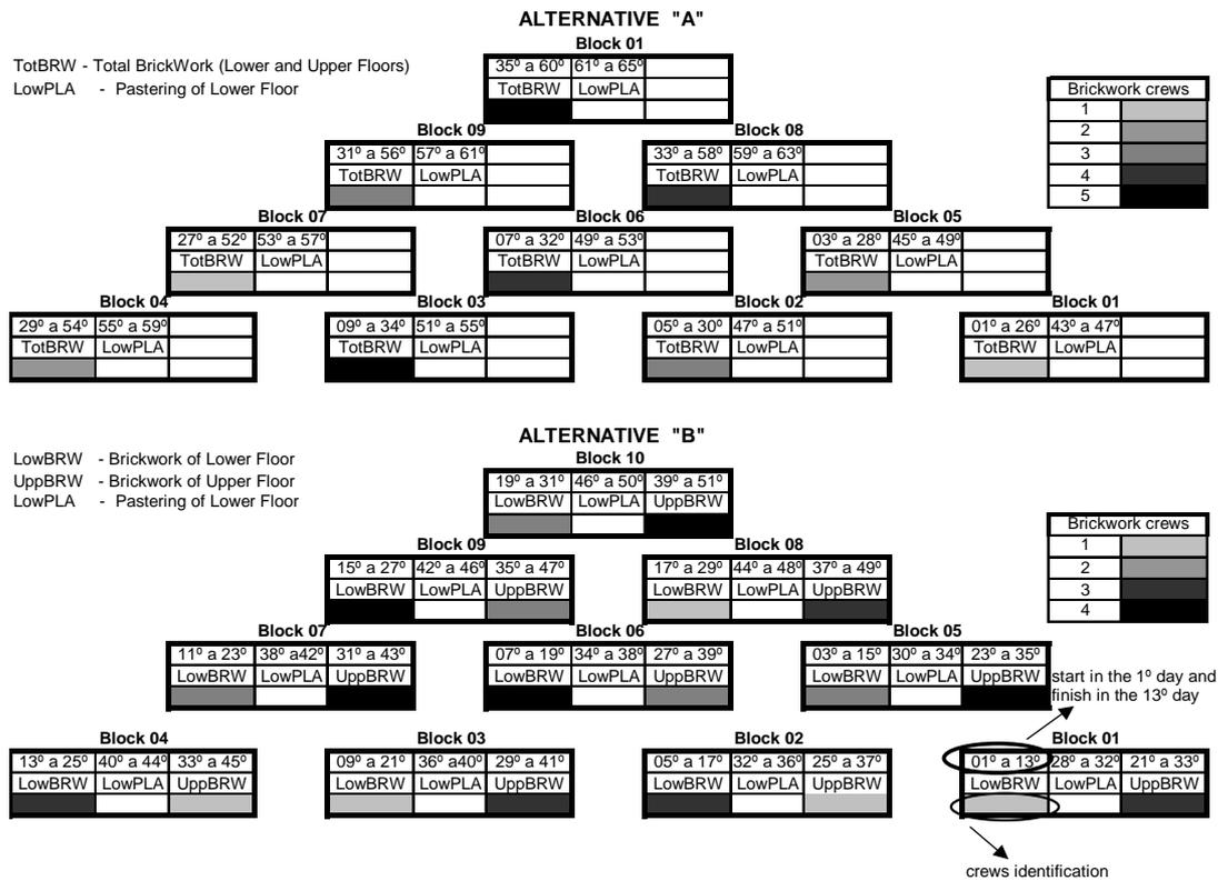
Figure 4: Work Flows of the Brickwork and Internal Plastering activities
