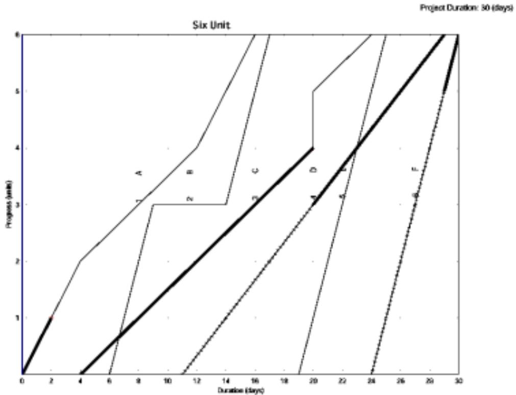
Figure 3. RSM Graphical Schedule for the Six-unit Project
