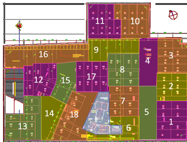
Figure 2: division of garage floor into similar complexities batches
