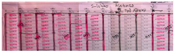
Figure 1: Image of how the actual installation schedule of precast concrete is documented and managed in Toriparkki construction project.
