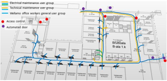
Figure 5: View on a mobile device showing access principles of a floor
