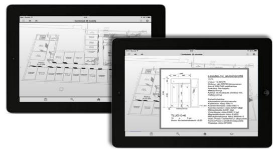
Figure 4: SMV on a mobile device showing the doors of a floor and an opened door specification.
