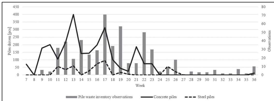
Figure 4: Piling Progress and Pile Waste Inventory Observations
