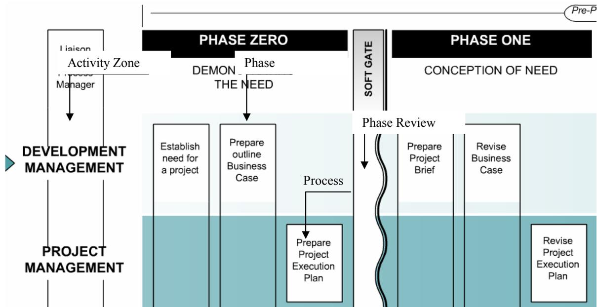
Figure 1: Process Protocol Framework
