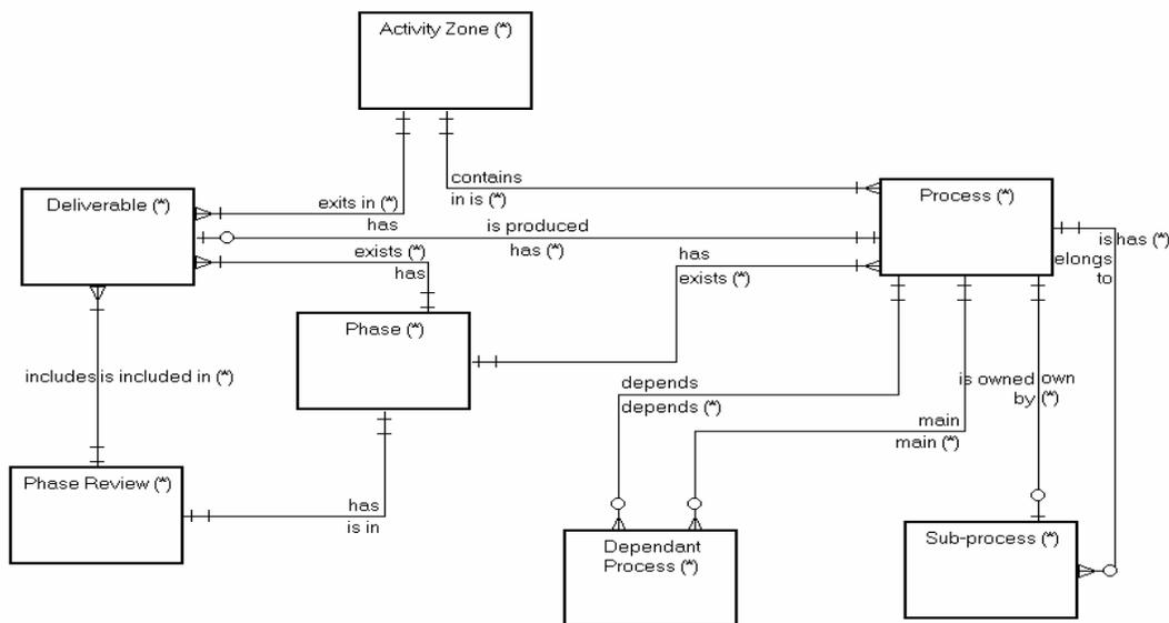
Figure 4: Entity Relationship Diagram for Process Protocol framework
