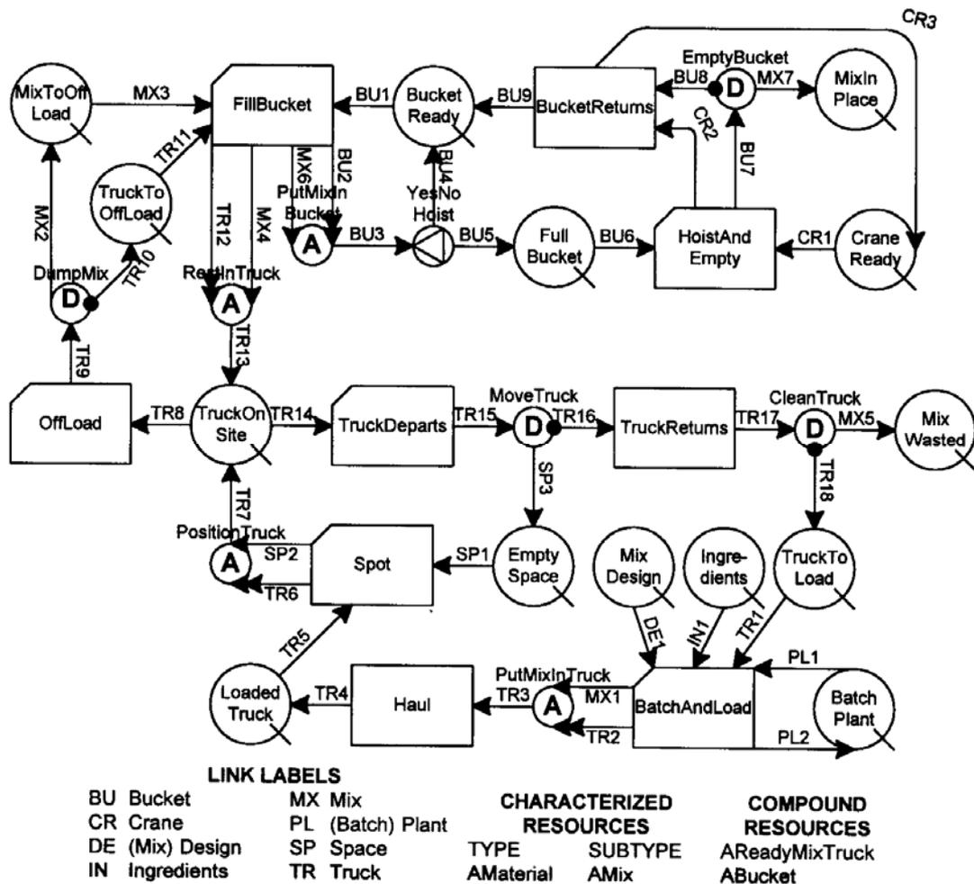
**Figure 3** Process model for concrete placement.
