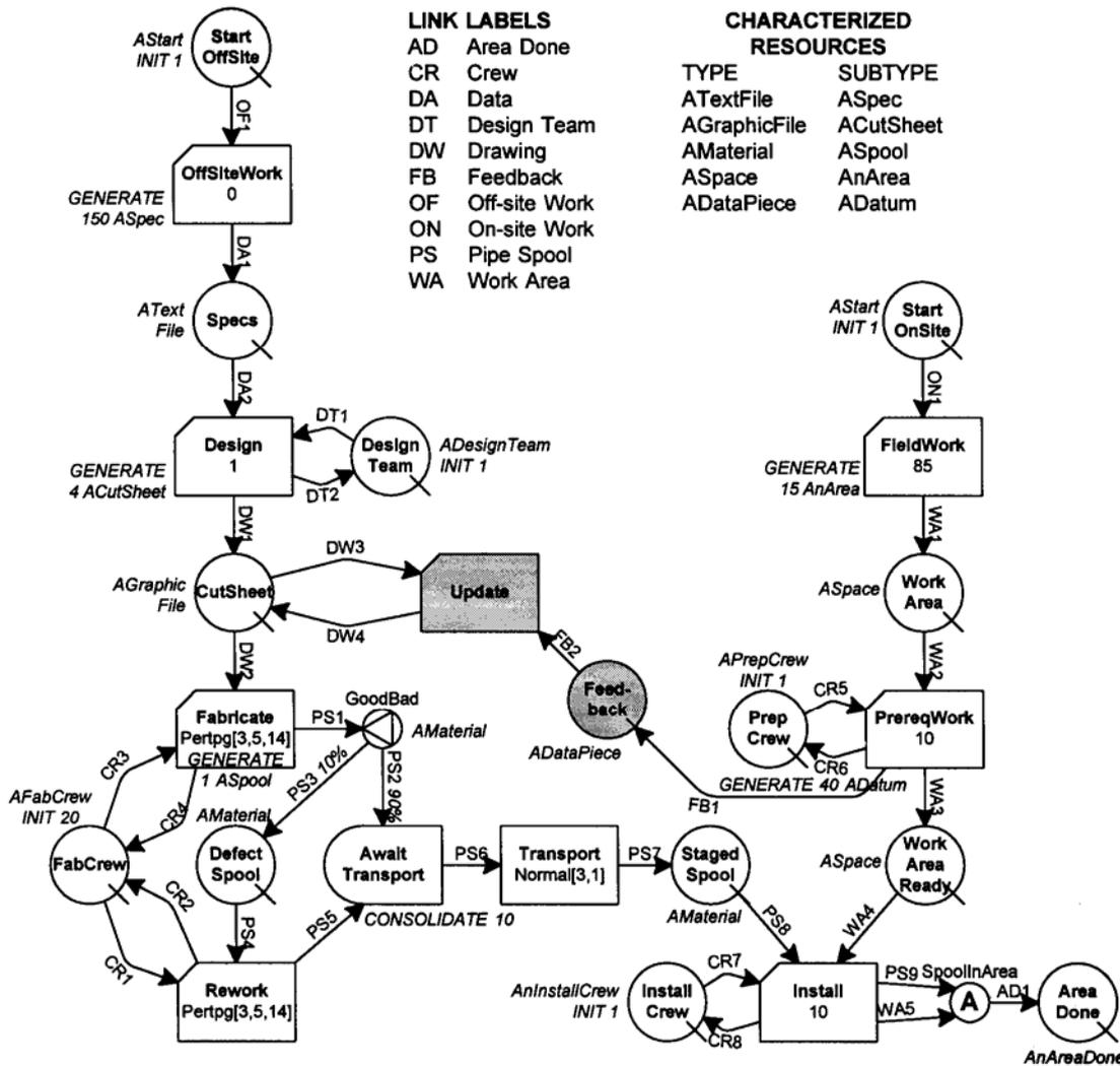
**Figure 1** Pipe-spool process model.
