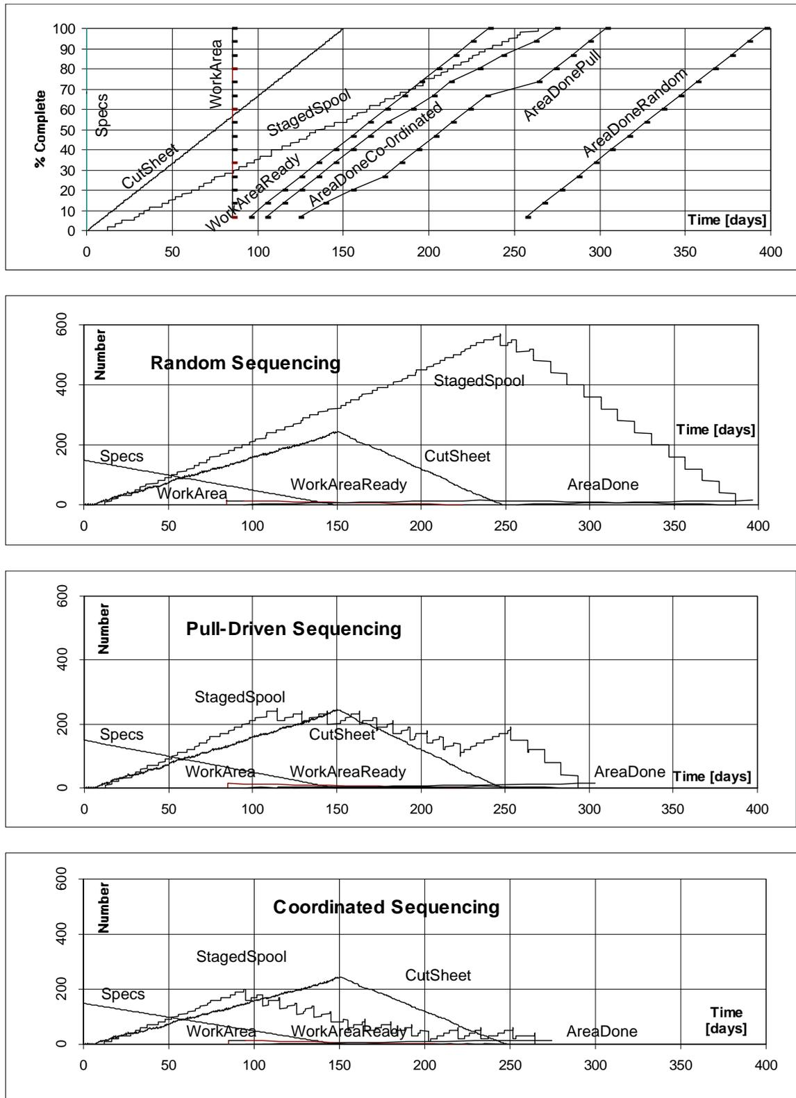
**Figure 2** % Complete vs. Time and Number of Resources vs. Time for Specs, WorkArea, CutSheet, StagedSpool, WorkAreaReady, and AreaDone Queues for Random, Coordinated, and Pull-Driven Sequencing.
