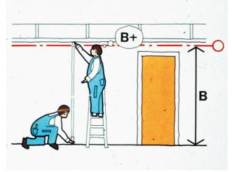
Figure.5: Tolerances in Construction meant that components sometimes lay outside their own 'basic' space.
