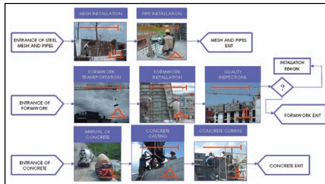
Figure 02: General outline of the experimental modelling system
