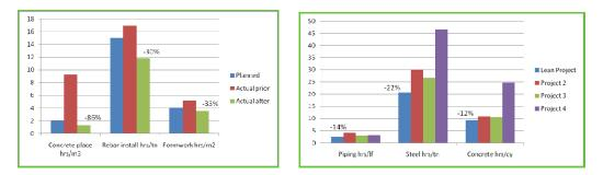
Figure 1: Unit production rate comparison within a project (planned, before, and after lean implementation)
