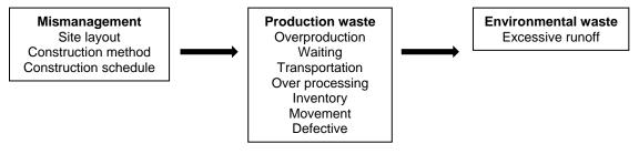
Figure 4: Mismanaged CM elements with Production and Runoff Waste
