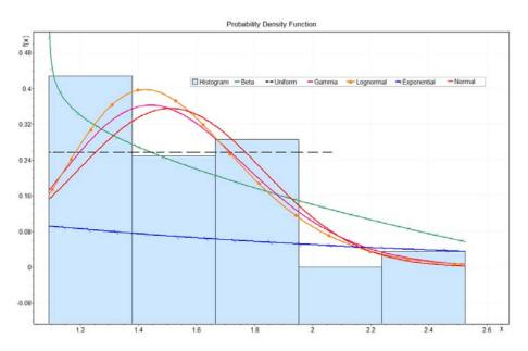
Figure 4: Probability Density Function of exterior wall productivity rate
