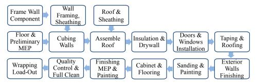
Figure 1: Production tasks layout of a modular building
