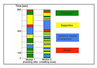
Figure 2: Crew Balance Chart for two workers, initial operation
