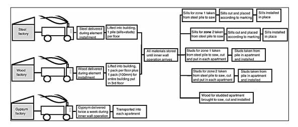
Figure 3: Process Map for all materials, initial operation
